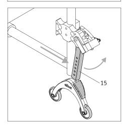
• Once the wheels are fitted, you can return the anti-tippers to their starting position. To do this, push the wheelchair forwards and at the same time push back the holding rod [73] using your foot.
