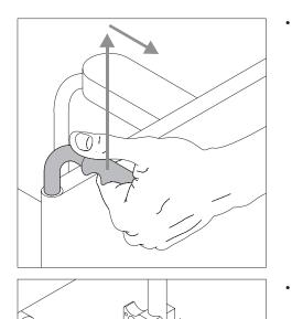
Whilst doing so, pull the wheelchair by its handles a little upwards and to the rear until the wheelchair has been raised and the anti-tippers click into a fixed position.
