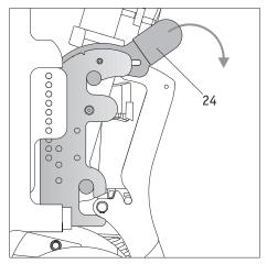
• If both bolts [3 and 4] are in their receivers [22 and 23] then you have to push down hard on the lock [24] on both sides in order to secure the viamobil to the wheelchair.
