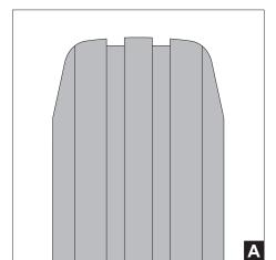
Your viamobil is an extremely low-maintenance device. No part of the drive is subject to noteworthy wear and tear with the exception of the tyres. The tyres are not to be used if they have reached their wear limit in order to be able to safely utilise the drive and braking power of your viamobil at all times.
