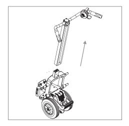
• Remove the hand grips from the drive unit, as shown in the figure.
