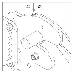
Your viamobil can only be started up when the bolts are correctly located in their receivers and secured by locks on both sides of the wheelchair.
