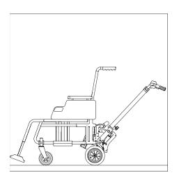
Push your viamobil from behind underneath the wheelchair, whereby the lower bolt [3] is initially inserted into the lower receiver [23] of the bracket on both sides.
