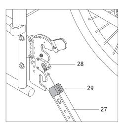
• Insert the receiver shoe [29] on the anti-tipper [27] into the fork opening [28].
