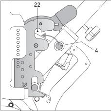
• If the lower bolt [3] is in the lower receiver [23], the viamobil has to be tilted forwards as shown in the figure so that the upper bolt [4] is inserted into the upper receiver [22] of the bracket on both sides.
